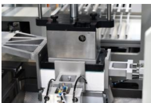
Punching with counterpressure
